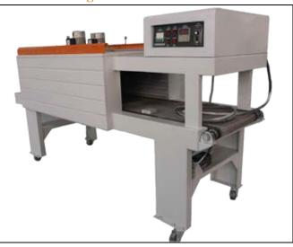
This machine can wrap the shrink film around the packed products, then heating to shrink and enswathe the packed parts. It can display the products' appearance completely to enhance the aesthetic effect and value of the commodities. Meanwhile it can get better sealing, prevent moisture and pollution, also can reduce the exterior impact on the products. This machine adopts Quartz far-infrared tube as heating source to save more than 15% electricity.
